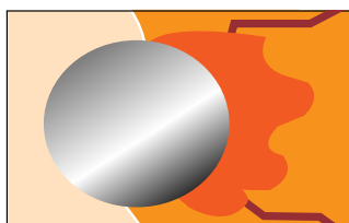
Cracking and spalling will ultimately occur.
